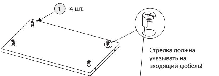
**Шаг 8** Установка планок монтажных
