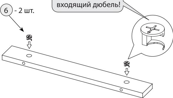
**Шаг 3** Соединение стенки нижней и цоколя
