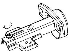
**Шаг 23** Установка доводчика на петлю
